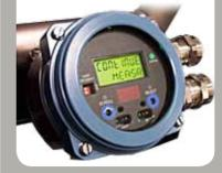
Meter verification can be initiated on the local operator interface. Additionally, the pass or fail results will be also accessible.
