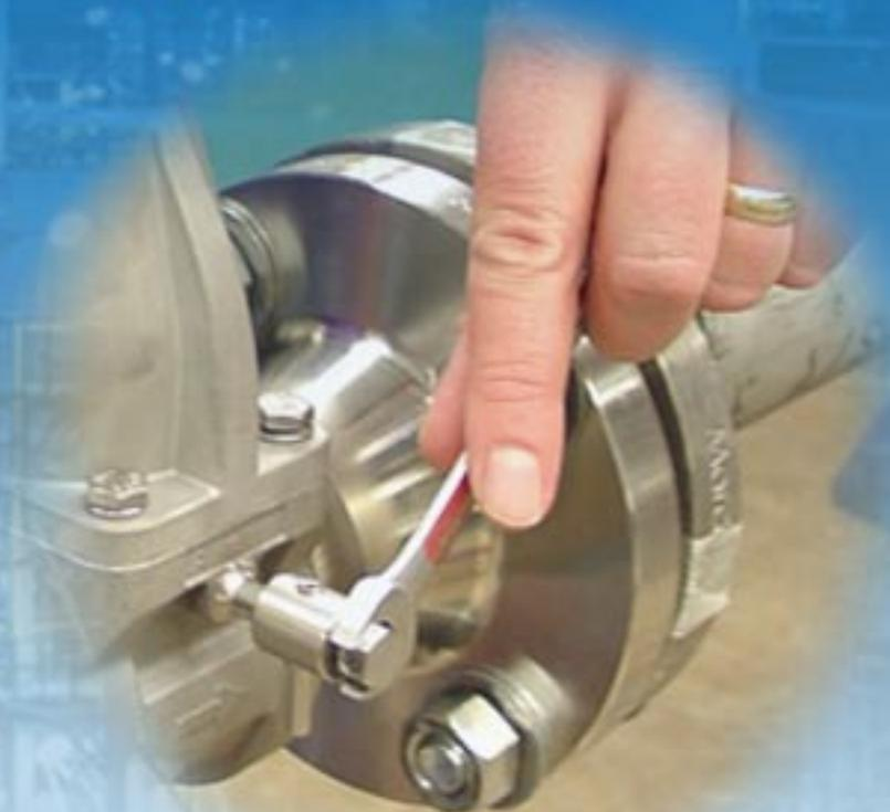
Rosemount CriticalProcess™ Vortex flowmeter enhances overall safety with a Vortex sensor isolated from the process.
