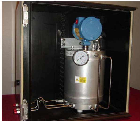
Micro Motion 3098 Gas Specific Gravity meter in enclosure
