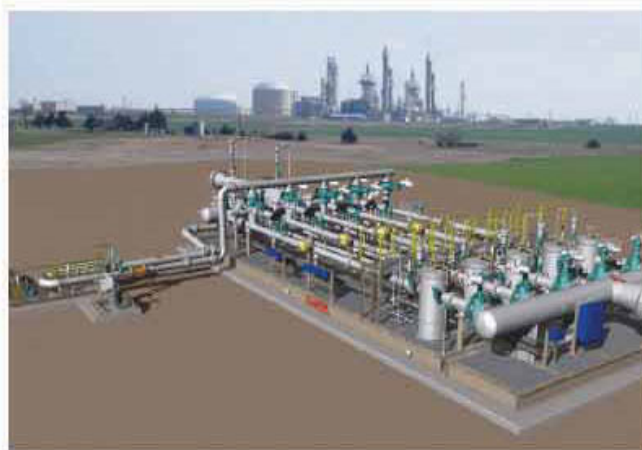
Figure 4. The Daniel skid design software creates a 3D image of the metering station skid.
