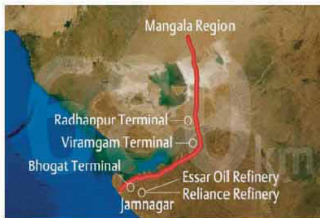
Figure 2. A 600 km heated, insulated pipeline, the longest of its kind in the world, carries heavy, waxy crude from wells in the Thar desert to refineries on India's western coast.
