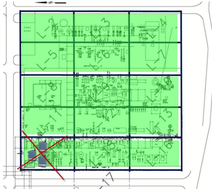
Figure 6-4. Process with Three WirelessHART Networks and Poor Gateway Placement
