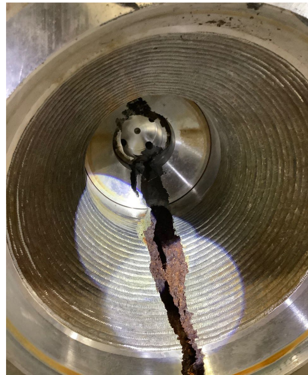
Example of injection pump min flow valve damage
