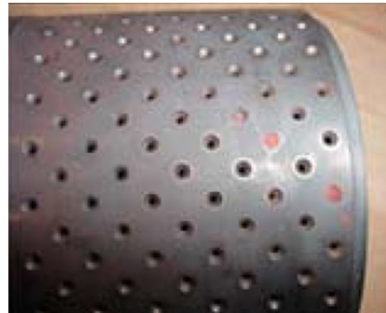
Example of Particulate Plugging Cage
