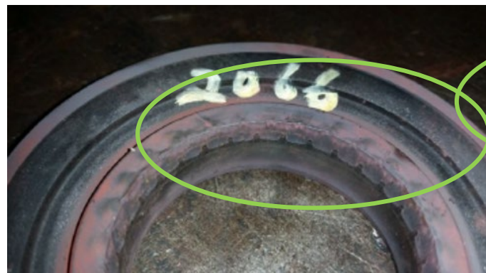
Gear Tooth Effect Damage on Plug & Seat
