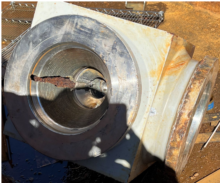
Example of injection pump min flow valve damage
