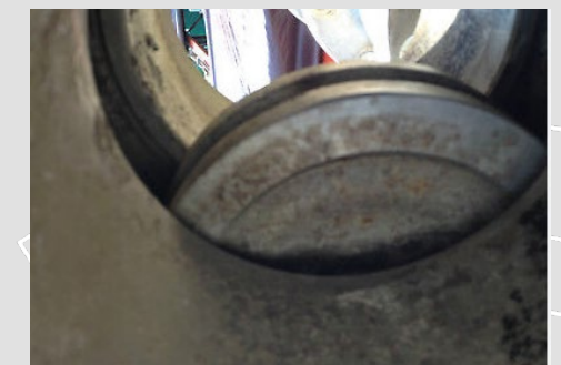
Typical Double Disc Gate valve failure
